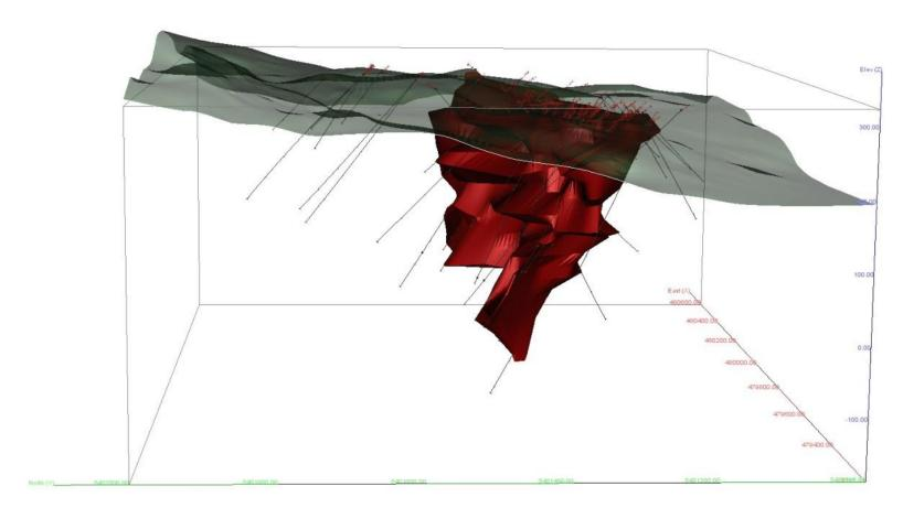
Plan view showing Isometric view looking east showing mineralized solid in red, surface topography in grey and drill hole traces.
