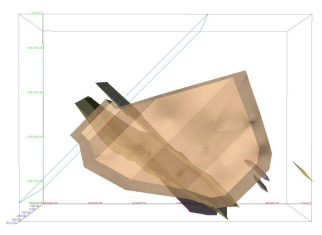
Plan view showing modelled dykes cutting through the mineralized solid.
